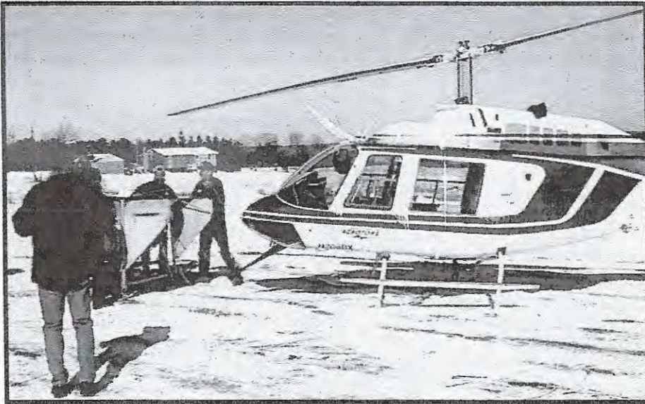
Ground crew at the landing zone prepares the sling bucket for loading and calibrating, prior to the actual sowing of white pine seed and fertilizer (March 8, 1999 - DCNR photo by John Bearer)
