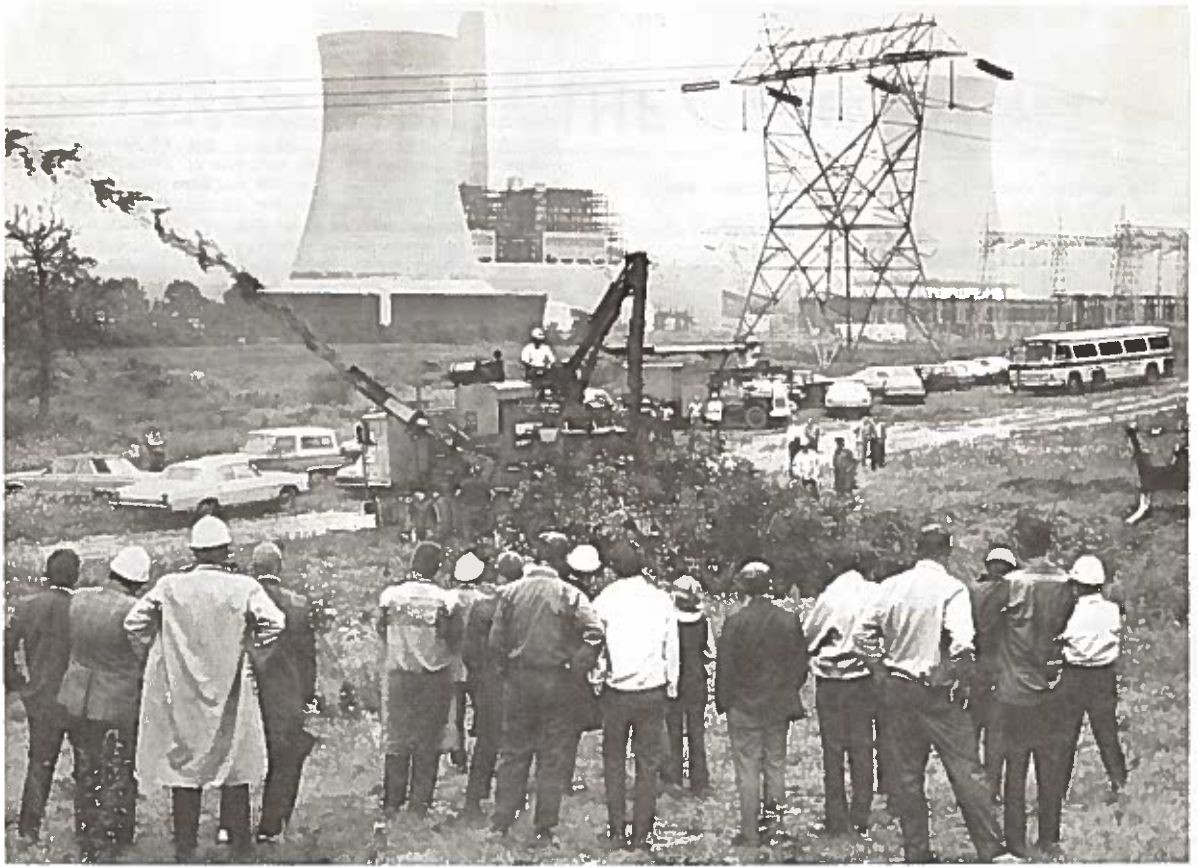
Members of the field trip group watch Penn Line's Metro chipper in action. The mobile mounted chipper features an integral boom-type feeder and is capable of handling trees up to 16 inches in diameter
